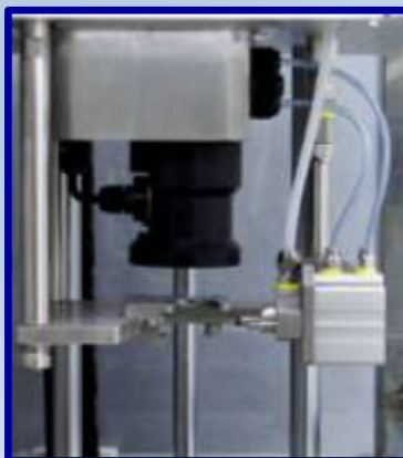
SSA-PLUS-P Neck piercing solution - micro-leakage can also be detected accurately
