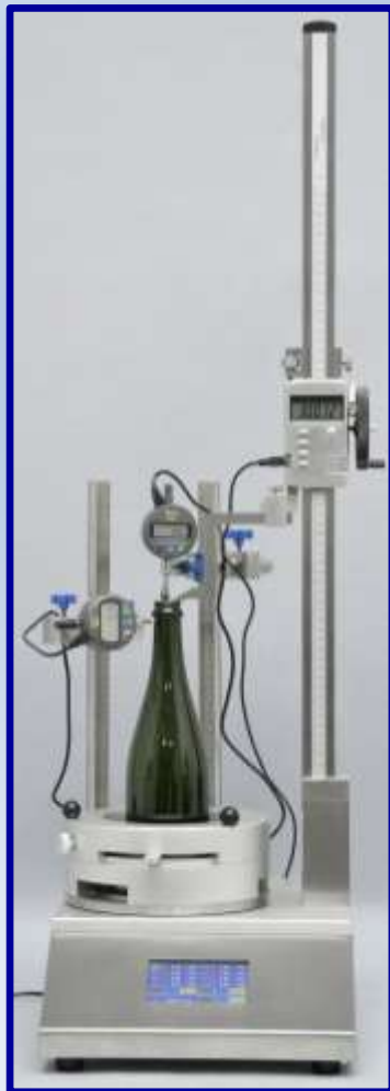
UBPT-3 with 3 measuring heads (for mouth clearance, perpendicularity & height) and integrated double automatic calculators
