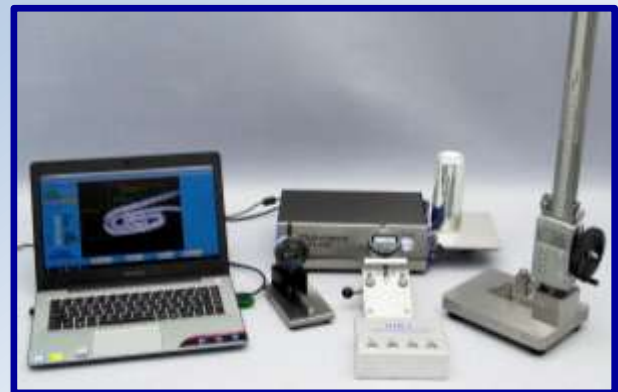
SeamCheck Plus is able to connect with optional gauges through DTB-1
