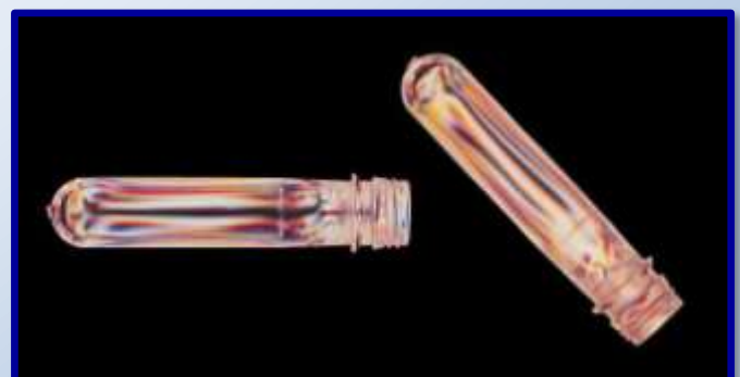
Parallel view and 45° view of preform by PL-P
