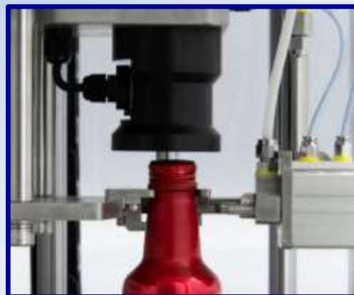
SSA-PLUS-P Neck piercing solution - micro-leakage can also be detected accurately
